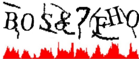
Fig. 3. Vertical histogram segmentation.
